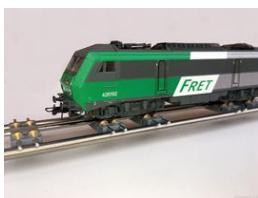
You have purchased an M2R test bench and I hope you are satisfied with it. It is particularly suitable for testing locomotives, adjusting analog and digital equipment, but also for demonstration.
